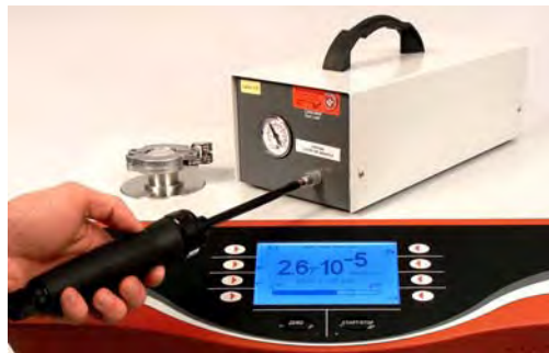
Fig. 6-81 Sniffing external test leak
