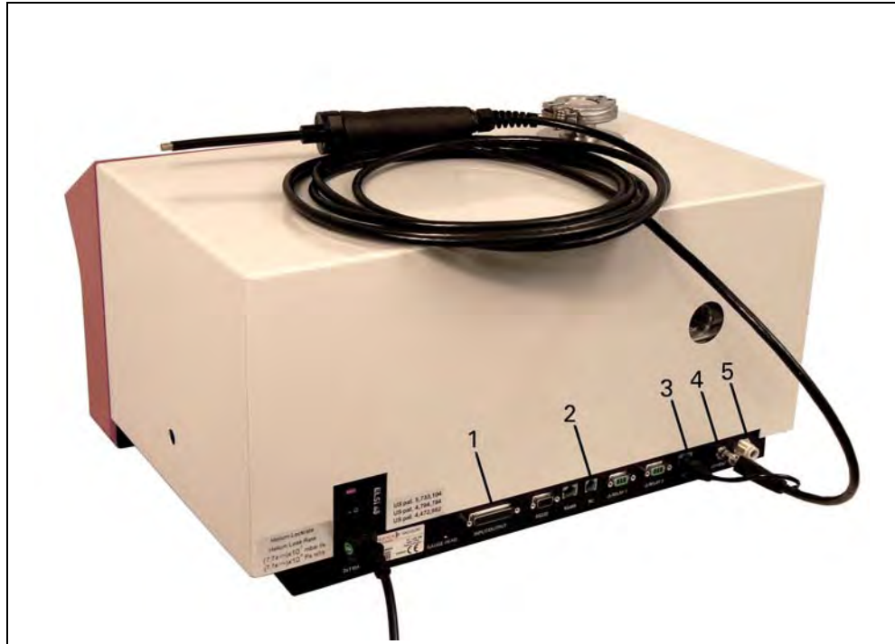
Fig. 5-2 Connections for sniffing probe
