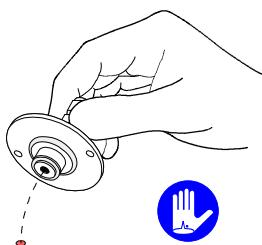
**4** Tilt the gas inlet in order for the orifice to drop out.
